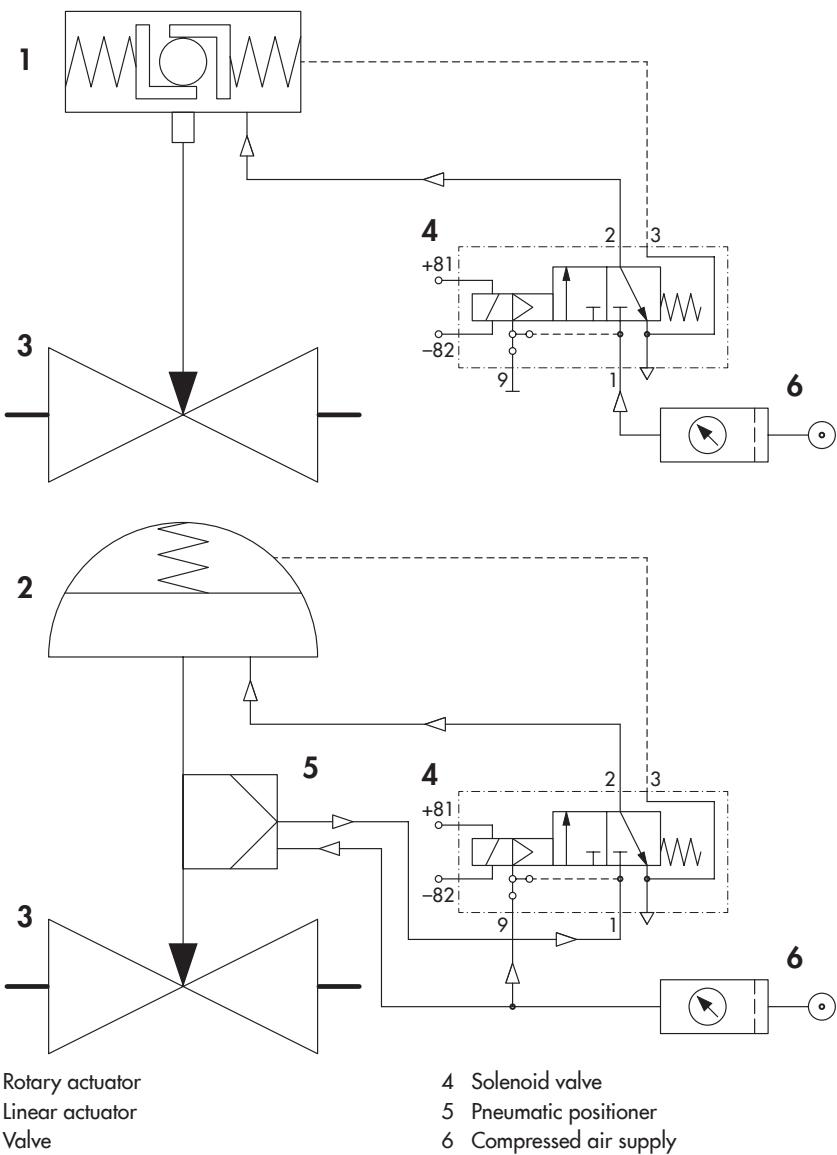
**Fig. 1:** Functional diagram showing emergency venting in actuators for on/off and throttling service
